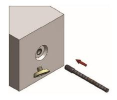
After removal of the shuttering system and removal of the fixing plate, the TSE coupler can be inserted and hand tightened.
