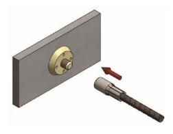
Thread the coupler onto the fixing plate attached to the shuttering system.
